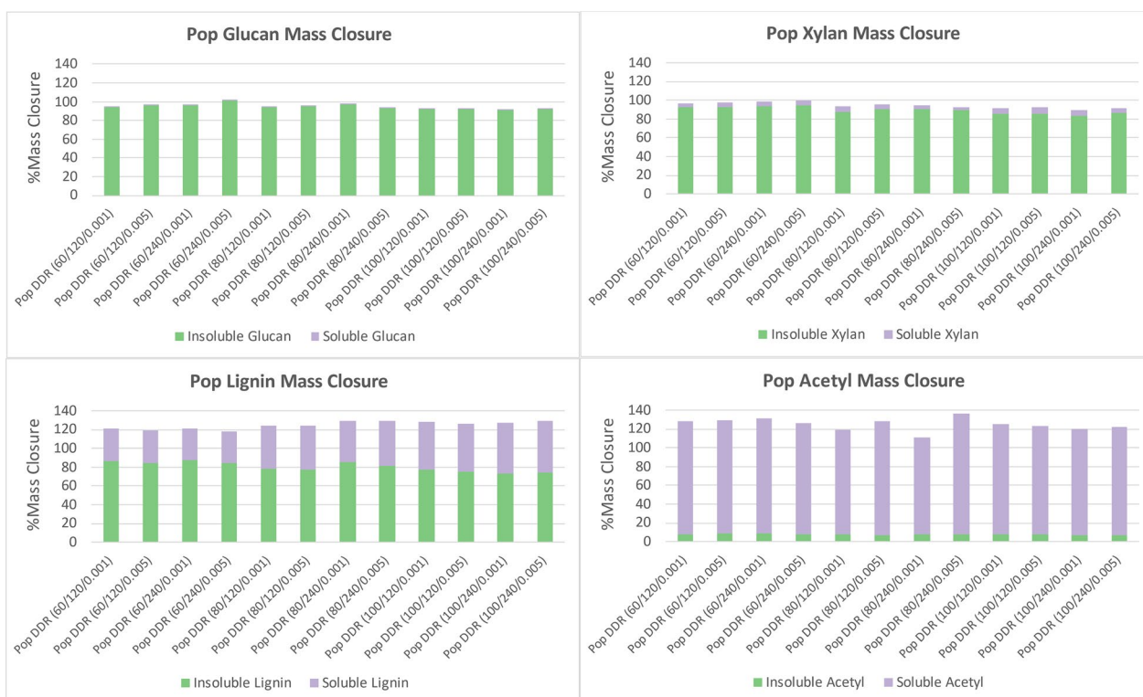
Fig. 3 Poplar (Pop) deacetylation mass closure of glucan (top left), xylan (top right), lignin (bottom left), and acetyl (bottom right). Lignin conversion yield to black liquor was likely overestimated due to the lack of an accurate quantifying method. Acetyl conversion yield was high due to under quantifying acetyl in the raw feedstock. The acetyl was nearly all removed from the insoluble solids fraction. Lignin was removed more when the concentration of sodium hydroxide was increased, but significantly less than corn stover. Most of the glucan and xylan, remain with the insoluble solids fraction. X/Y/Z represents NaOH conc (g/kg)/residence time (min)/disc-refining gap (in.)
