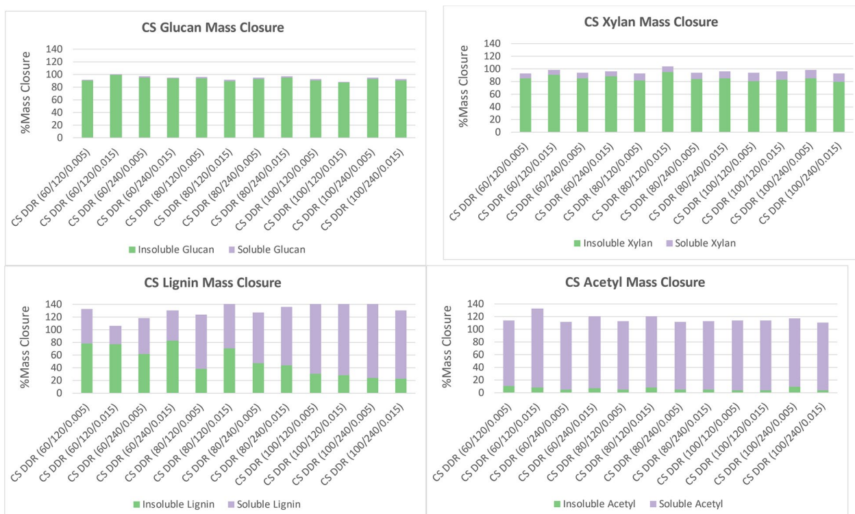
Fig. 2 Corn stover (CS) deacetylation mass closure of glucan (top left), xylan (top right), lignin (bottom left), and acetate (bottom right). Lignin conversion yield to black liquor is likely overestimated due to the lack of an accurate quantifying method. Acetyl conversion yield is high due to under quantifying acetyl in the raw feedstock. Acetyl is nearly all removed from the solids fraction. Lignin is removed more when the concentration of sodium hydroxide is increased. Most of the glucan and xylan, remain within the insoluble solids fraction. X/Y/Z represents NaOH conc (g/kg)/residence time (min)/disc-refining gap (in.)
