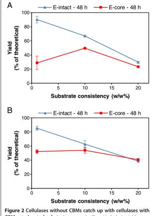
**Figure 2** Cellulases without CBMs catch up with cellulases with CBMs at elevated substrate concentration. Hydrolysis yield as a function of substrate consistency after 48 hours hydrolysis of (A) Avicel and (B) pre-treated wheat straw at 45°C with the enzyme mixtures containing intact (blue) or core (red) enzymes (Table 1).
