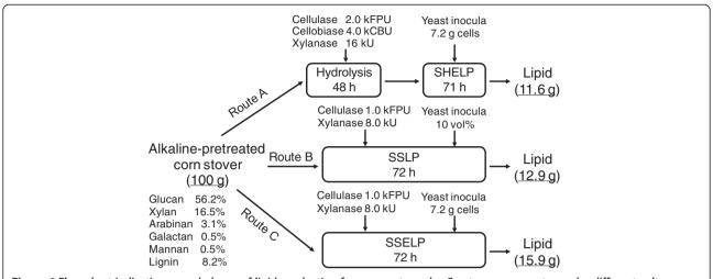
**Figure 4** Flow chart indicating mass balance of lipid production from corn stover by *Cryptococcus curvatus* under different culture modes. CBU, cellobiase unit; FPU, filter paper unit; SHELP, separated hydrolysis and enhanced lipid production; SSELP, simultaneous saccharification and enhanced lipid production; SSLP, simultaneous saccharification and lipid production.
