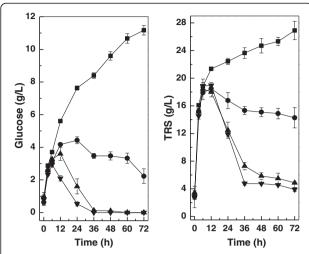
**Figure 2** Sugar evolution profiles of the simultaneous saccharification and lipid production process by *Cryptococcus curvatus* in different solutions. Square, potassium phosphate buffer; circle, nutrient solution plus 0.1 g/L (NH<sub>4</sub>)<sub>2</sub>SO<sub>4</sub>; triangle, nutrient solution plus 0.5 g/L (NH<sub>4</sub>)<sub>2</sub>SO<sub>4</sub>; inverted triangle, nutrient solution plus 1.0 g/L (NH<sub>4</sub>)<sub>2</sub>SO<sub>4</sub>. TRS, total reducing sugars.
