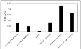
**Fig. 2** Process contribution to global warming. Six main units of the sugar process are shown with their corresponding GW impacts (measured in  $CO_2$  equivalents/kg)
