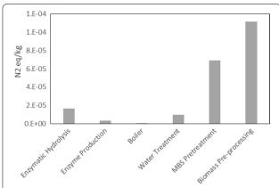
**Fig. 3** Process contribution to eutrophication. Six main units of the sugar process are shown with their corresponding eutrophication impacts (measured in Nitrogen equivalents/kg)
