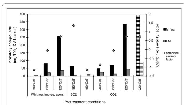
**Figure 4** Concentration of inhibitory byproducts in the hydrolysate obtained after the steam pretreatment of sugar cane leaves at different conditions. The pretreatment combined severity factor for each set is also shown. Striped columns correspond to cut, not milled, sugar cane leaves. For two of the samples the concentration of furfural was low and could not be evaluated in the high performance liquid chromatography (HPLC) chromatogram due to overlap with other peaks.
