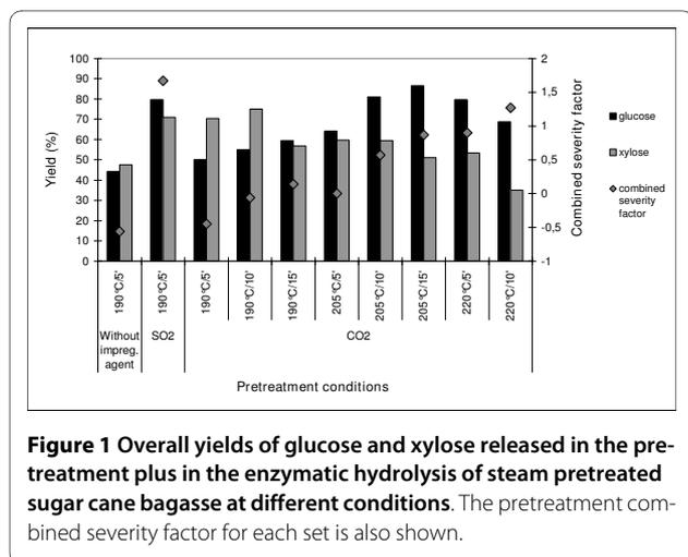
**Figure 1** Overall yields of glucose and xylose released in the pretreatment plus in the enzymatic hydrolysis of steam pretreated sugar cane bagasse at different conditions. The pretreatment combined severity factor for each set is also shown.
