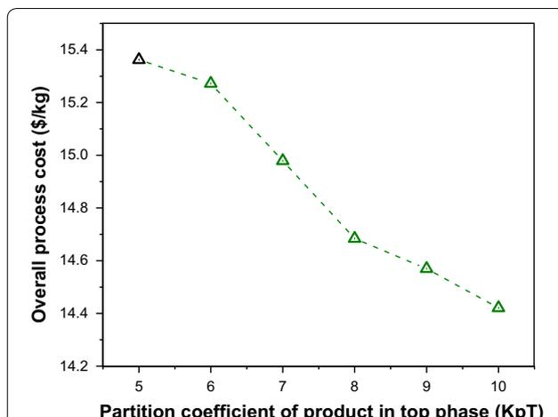
**Fig. 18** Overall process cost as a function of partition coefficient of product in the top phase (KpT). The result with nominal KpT value is shown by the black marker at (5, 15.36)
