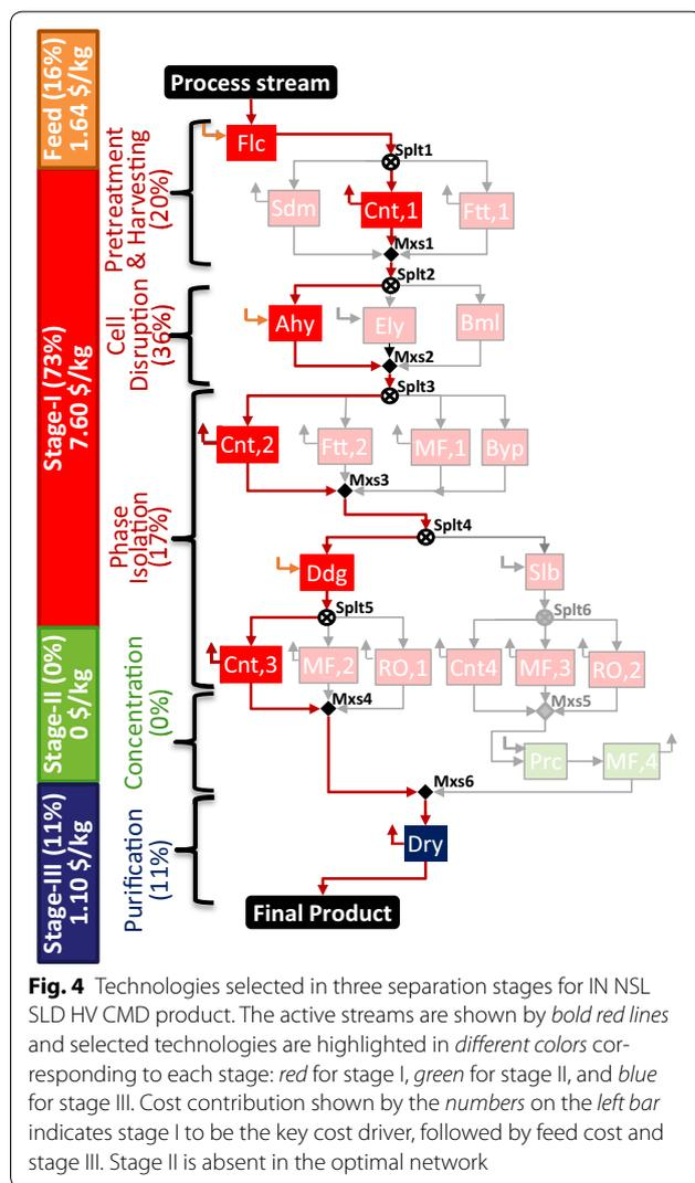
centrifugation (Cnt,1) for cell harvesting, acid hydrolysis (Ahy) for cell disruption, centrifugation (Cnt,2) for initial phase separation, and differential digestion (Ddg) for product-rich phase formation, followed by centrifugation (Cnt,3) to separate the solid product from the digested NPCM and other liquid phase components. Stage II is
