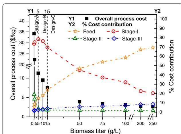
**Fig. 13** Overall process cost and contributions by feed and separation stages with varying biomass titer. Axis Y1 represents the overall process cost per unit product. Axis Y2 represents the cost contribution of the feed and three separation stages. The vertical dotted lines at 5 and 15 g/L represent the change in optimal separation network design
