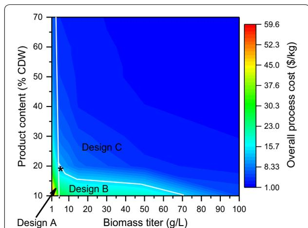
**Fig. 16** Overall process cost as a function of biomass titer and product content. The change in optimal separation network design is denoted by the white lines and the details of the selected technologies and active stream in designs a, b, and c are the same as those represented in Fig. 14. The base case (5 g/L, 20% CDW) is denoted by the black asterisk
