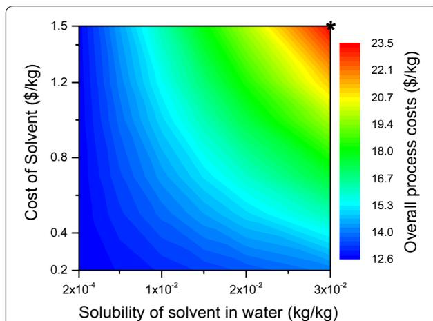
**Fig. 19** Overall process cost as a function of solubility of solvent and cost of solvent. The nominal values assumed for the three parameters (Kp—1.2 (not shown), cost of solvent—1.5 \$/kg (Y axis), and solubility of solvent in water—0.03 kg/kg (X axis) and the corresponding overall process cost are shown by the black asterisk
