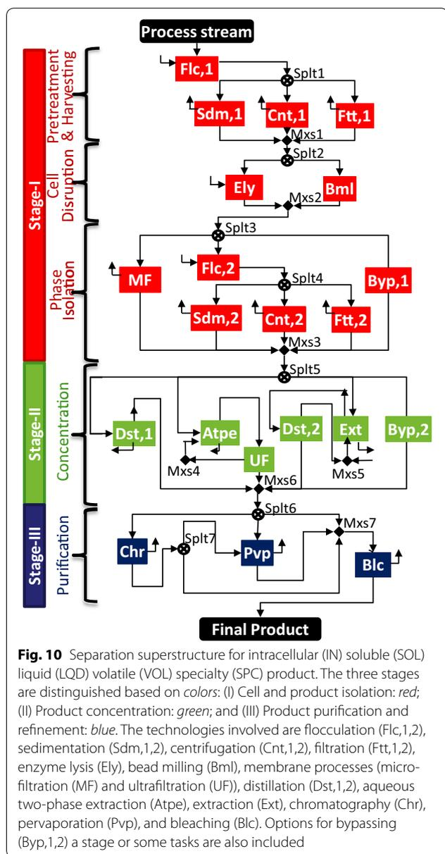
purification and refining of the product, technologies like chromatography, pervaporation, and bleaching are available in stage III. Some basic input parameters for the case study are presented in Table 7.
