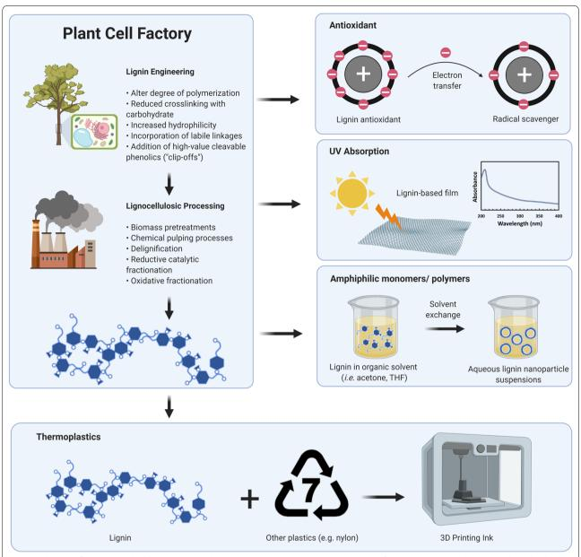
**Fig. 5** Schematic flow diagram highlighting that both plant engineering and down-stream lignin fractionation approaches can and need to be combined to isolate high purity lignin fractions with preferred structural characteristics for industrial utilization. Properties inherent in the lignin can be exploited for functional materials that include, but are not limited to, antioxidants, UV absorptive films, self-assembled nanoparticles, and melt processable lignin for 3D printing
