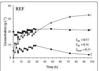
Figure 1 Measured concentrations during duplicate reference fed-batch simultaneous saccharification and co-fermentation (SSCF) of wheat straw (8%-11% WIS) showing glucose (black circle), xylose (black square) and ethanol (black triangle). No enzyme feed was used; all enzymes were added initially. The mean standard deviation ( $\overline{s}$ ) is given for the concentration profile and illustrated graphically at the right end of each profile.
