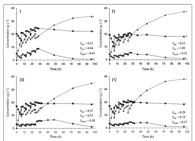
Figure 2 Measured concentrations during duplicate fed-batch SSCF of wheat straw (8%-11% WIS) showing glucose (black circle), xylose (black square) and ethanol (black triangle) when using different enzyme feed strategies: (I) Feed profile A, (II) Feed profile B, (III) Feed profile C, (IV) Feed profile D. The mean standard deviation ( $\overline{s}$ ) is given for the concentration profile and illustrated graphically at the right end of each profile.
