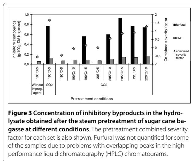
**Figure 3** Concentration of inhibitory byproducts in the hydrolysate obtained after the steam pretreatment of sugar cane bagasse at different conditions. The pretreatment combined severity factor for each set is also shown. Furfural was not quantified for some of the samples due to problems with overlapping peaks in the high performance liquid chromatography (HPLC) chromatograms.
