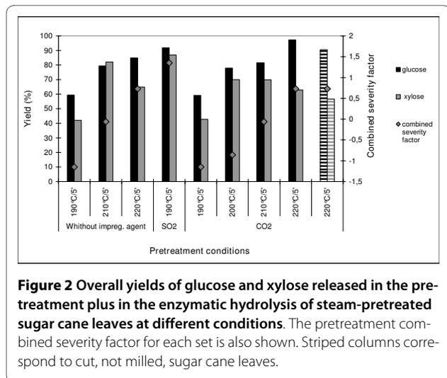
**Figure 2** Overall yields of glucose and xylose released in the pretreatment plus in the enzymatic hydrolysis of steam-pretreated sugar cane leaves at different conditions. The pretreatment combined severity factor for each set is also shown. Striped columns correspond to cut, not milled, sugar cane leaves.
