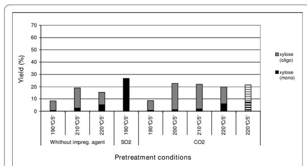
**Figure 6** Monomeric and oligomeric xylose (except for SO<sub>2</sub> impregnation) yields in the hydrolysate obtained after the steam pretreatment of sugar cane leaves at different conditions. Stripped columns correspond to cut, not milled, sugar cane leaves.
