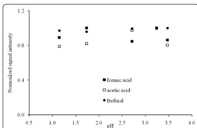
**Figure 1** Normalised average headspace signal intensities for formic acid, acetic acid and furfural as a function of pH (in phosphate buffer). Data are normalised to the maximum signal intensity observed for each compound. Each value is the mean of three replicate measurements, and from this the percentage coefficient of variance (%CV = (standard deviation  $\div$  mean)  $\times$  100) for each compound was calculated as formic acid (17.8%), acetic acid (12.5%) and furfural (4.4%).
