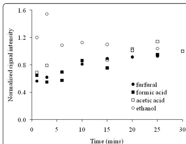
**Figure 2** Average headspace equilibration profiles of furfural, acetic acid, formic acid and ethanol. The headspace signal intensity was normalised to the signal at 30 minutes. Each data point is the average of two replicate analyses. %CV values were ethanol (15.4%), formic acid (16.3%), acetic acid (17.5%) and furfural (4.7%).
