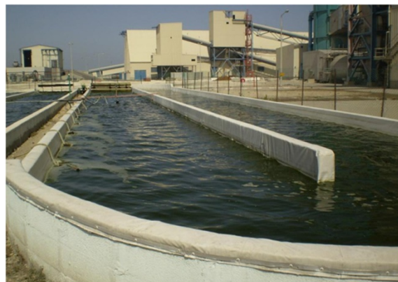
Figure 1 Cultivation of Nannochloropsis sp. microalgae using seawater in open systems at the Seambiotic company, Israel, 2009.
