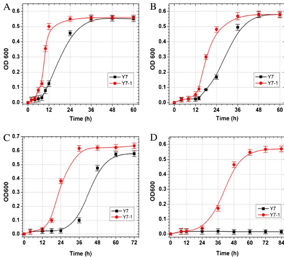
**Figure 1** Cell growth of parental strain Y7 and adapted strain Y7-1 as measured at OD<sub>600</sub> on the defined medium containing 10 Mm (A), 20 mM (B), 30 mM (C) and 40 mM (D) furfural.
