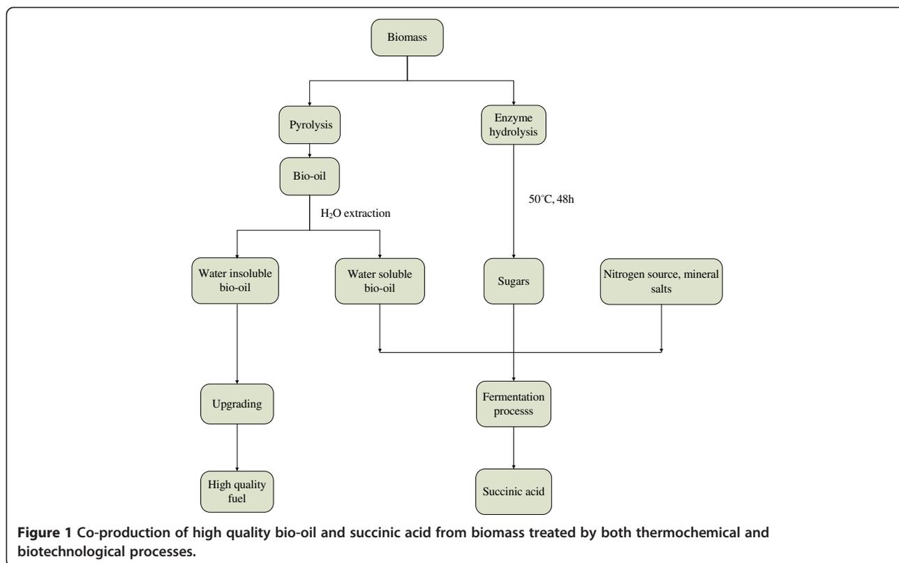
**Figure 1** Co-production of high quality bio-oil and succinic acid from biomass treated by both thermochemical and biotechnological processes.
