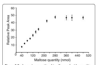
Figure 3 Peak area is proportional to oligosaccharide quantity. Maltose was derivatised with APTS and the resulting peak area compared to an internal standard. Bars represent s.d, n=3.
