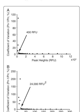
Figure 2 Reproducibility of quantitation of oligosaccharides in parallel capillaries. (A) Peak height measurements are highly reproducible. (B) Peak area measurements are highly reproducible. Below approximately height 400 RFU or area 20000 RFU<sup>2</sup>, the measurements are less reproducible
