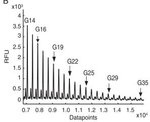
**Figure 1 Separation of APTS-labelled oligosaccharides by CE in an ABI 3730xl DNA sequencer. (A)** Electropherogram trace (50 min) of APTS labelled hydrolysed dextran and β-1,4-xylo oligosaccharides DP1 to DP6. **(B)** Large DP hydrolysed dextran oligosaccharides can be resolved by extending the electrophoresis time to 90 minutes. RFU, relative fluorescence units; G, Glucose; X, Xylose.
