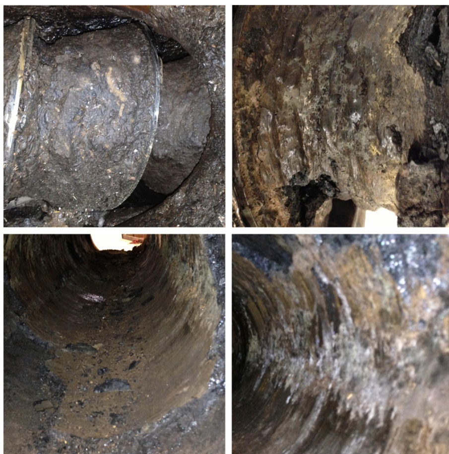
Figure 4 Images of carbonaceous deposits observed on reactor augers and walls.
