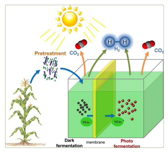
Simultaneous hydrogen and ethanol production from cascade utilization of mono-substrate in integrated dark and photo-fermentative reactor
