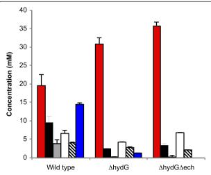
**Figure 2 Fermentation products of** *C. thermocellum*. The wild-type,  $\Delta hydG$ , and  $\Delta hydG\Delta ech$  strains grown on minimal medium with 5 g/L cellobiose. Red bar, ethanol; black bar, acetate; gray bar, lactate; white bar, formate; diagonal line bar, total amino acids; blue bar,  $H_2$ .  $H_2$  concentration is reported as mmol gaseous  $H_2$  per L liquid medium to facilitate comparison to soluble products. Error bars represent one standard deviation.
