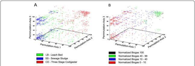
**Fig. 2** 3D plots of chemical parameters. COD, TOC, total nitrogen contents (N), conductivity, TVFA, TS, VS, pH, and produced volume of biogas are plotted in a 3D representation in which the permutation of all determined parameters define axis X, Y, and Z. The underlying biogas facilities are highlighted correspondingly (a). Plotting the parameters without the biogas yield and colorizing the *dots* according to their biogas production rate gives the second plot (b)
