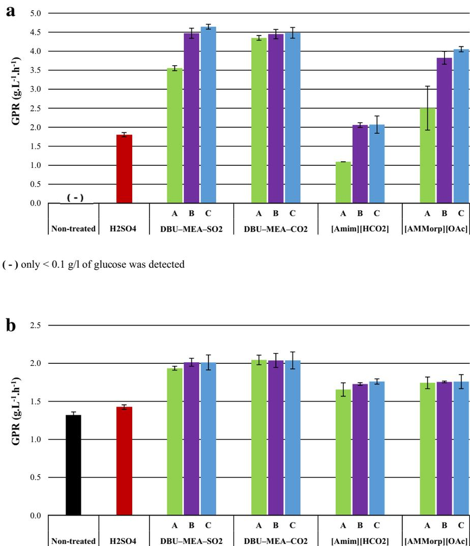
**Fig. 3** Glucose production rates (GPRs) during 4-h enzymatic hydrolysis of lignocellulose substrates. **a** Reed canary grass; and **b** Pine bark. Enzymatic hydrolysis experiments were performed with either non-treated or H<sub>2</sub>SO<sub>4</sub>-treated (SF 4.1), or (S)IL-treated lignocelluloses. (S)IL treatments were performed at (A) SF 2.5 (B) SF 3.7 and (C) SF 4.1
