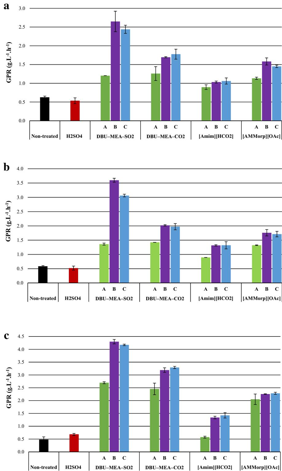
**Fig. 2** Glucose production rates (GPRs) during 4-h enzymatic hydrolysis of lignocellulose substrates. **a** Spruce wood; **b** Pine stem wood; **c** Birch wood. Enzymatic hydrolysis experiments were performed with either non-treated or H<sub>2</sub>SO<sub>4</sub>-treated (SF 4.1), or (S)IL-treated lignocelluloses. (S)IL treatments were performed at (A) SF 2.5 (B) SF 3.7 and (C) SF 4.1
