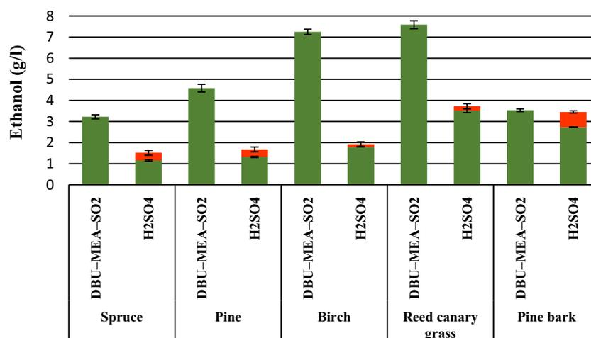
**Fig. 6** Ethanol produced from the fermentations of lignocellulose hydrolysates. Green bars represent ethanol produced from the enzymatic hydrolysates and red bars represent ethanol produced from the liquid fraction of acid pre-hydrolysis. Enzymatic hydrolysis experiments were performed with lignocellulose that were first treated with either H<sub>2</sub>SO<sub>4</sub> (SF 4.1) or with the SIL DBU-MEA-SO<sub>2</sub> (SF 4.1)
