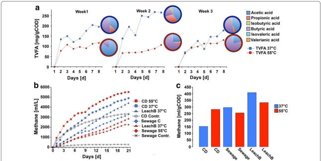
**Fig. 2** Chemical parameters during acidification and methane production: total amount of TVFA was monitored daily and samples obtained at the end of each acidification cycle were subjected to the determination of VFA spectra (**a**). Produced methane is shown as volume of methane per volume of sludge (**b**) and as volume of methane per mg of input COD (**c**)
