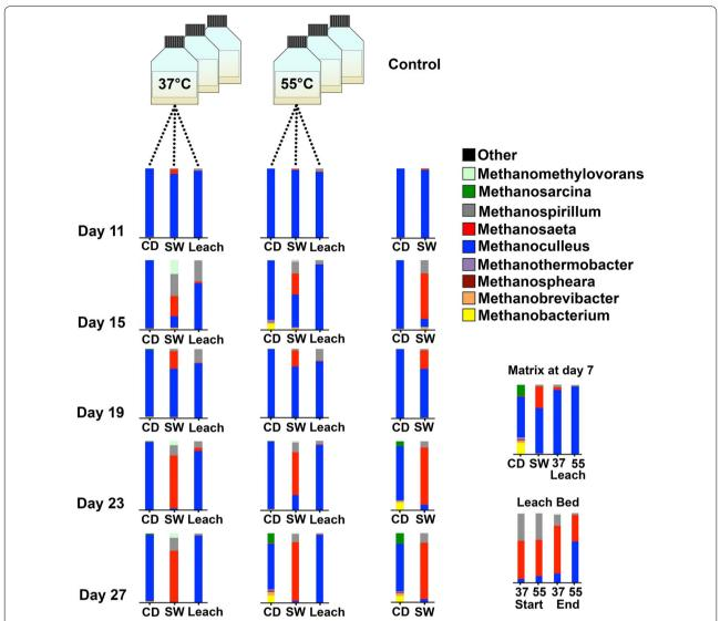
**Fig. 4** Archaeal community in the  $CH_4$ -stages: Time-dependent community behaviour at the genus level over 20 days for various  $CH_4$ -stages digesting hydrolysate from mesophile and thermophile acidification. All  $CH_4$ -stage measurements were performed at mesophilic temperatures. *CD* co-digester, *SW*—sewage, *Leach* Leachate
