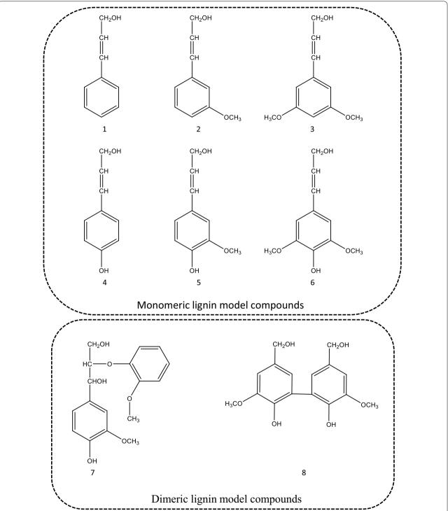
**Fig. 3** Lignin model compounds used in this study: (1) Cinnamic acid (H), (2) 3-methoxy cinnamic acid (G), (3) 3,5-dimethoxy cinnamic acid (S), (4) p-coumaric acid (H), (5) ferulic acid (G), (6) sinapic acid (S), (7) guaiacylglycerol β-guaiacyl ether (β-O-4 dimer), and (8) dehydrodivanillic alcohol (5-S' dimer)
