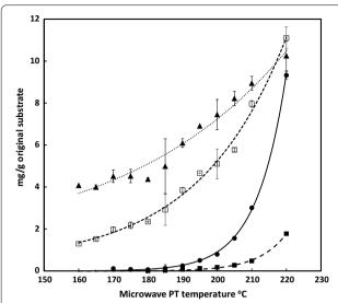
**Fig. 1** Effect of pretreatment severity on inhibitors released into liquor (mg/g original substrate). Symbols: Formic acid (filled triangle); 5-HMF (filled square); 2-FA (filled circle); Acetic acid (opened square) (n = 2)
