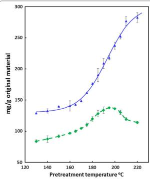
**Fig. 2** Effect of pretreatment severity on the enzymatic release of glucose (blue triangle) and xylose (green diamond) from wheat straw (n = 2)
