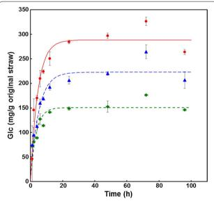
**Fig. 4** Time course of glucose release from wheat straw pretreated at 175 °C (green diamonds), 195 °C (blue triangles), and 210 °C (red circles) for 10 min, saccharified with excess cellulase (30 FPU/g original material); n=2
