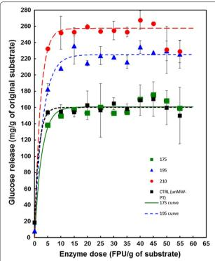
**Fig. 3** Effect of cellulase dose on the release of glucose from wheat straw pretreated at three different severities: Symbols: control (black squares); 175 °C for 10 min (green squares); 195 °C for 10 min (blue triangles); 210 °C for 10 min (red circles); n=2
