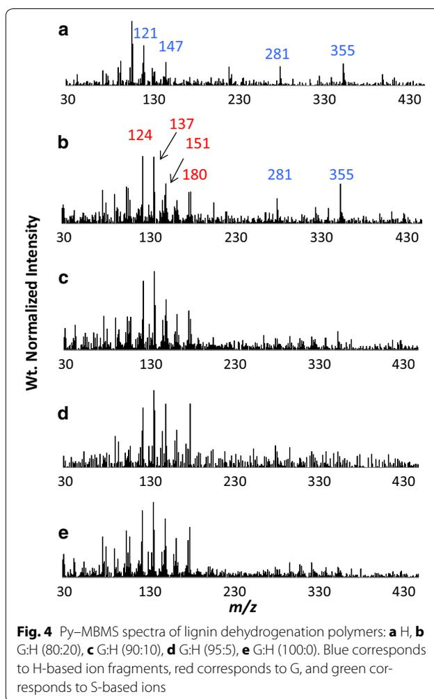
**Fig. 4** Py-MBMS spectra of lignin dehydrogenation polymers: **a** H, **b** G:H (80:20), **c** G:H (90:10), **d** G:H (95:5), **e** G:H (100:0). Blue corresponds to H-based ion fragments, red corresponds to G, and green corresponds to S-based ions
