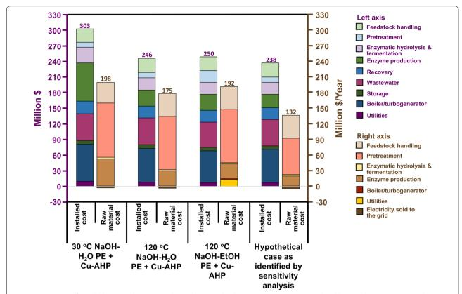
**Fig. 5** Comparison of installed costs and raw material costs between the three process scenarios considered by TEA. These scenarios are then compared to a "hypothetical case" 120 °C NaOH-H<sub>2</sub>O pre-extraction process that reduces H<sub>2</sub>O<sub>2</sub>, enzyme, and bpy loadings in concert. Note that raw material costs in this figure include the by-product revenue from electricity sales
