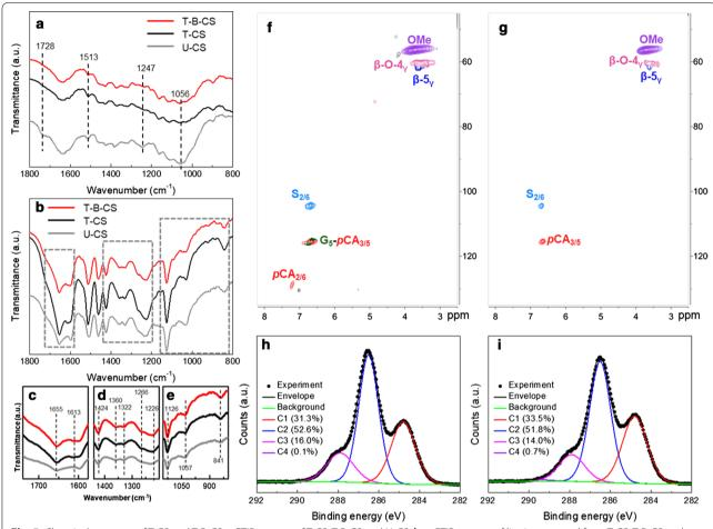
Fig. 5 Chemical structure of T-CS and T-B-CS. a FTIR spectra of T-CS, T-B-CS and U-CS, **b**-e FTIR spectra of lignin extracted from T-CS, T-B-CS and U-CS, **f** HSQC spectrum of lignin extracted from T-CS, and i XPS results for T-B-CS, h XPS results for T-CS, and i XPS results for T-B-CS
