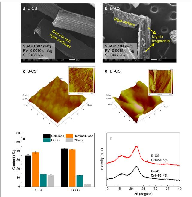
**Fig. 1** Morphology and composition of U-CS and B-CS. **a** SEM image of U-CS, **b** SEM image of B-CS, **c** AFM images of U-CS, **d** AFM images of B-CS, **e** composition of U-CS and B-CS, and **f** XRD patterns of U-CS and B-CS. Error bars shown in (**e**) are standard deviations of triplicate samples
