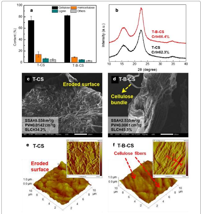
**Fig. 4** Composition and morphology of T-CS and T-B-CS. **a** Composition of T-CS and T-B-CS, **b** XRD patterns of T-CS and T-B-CS, **c** SEM image of T-CS, **d** SEM image of T-B-CS, **e** AFM images of T-CS, and **f** AFM images of T-B-CS. Error bars shown in (**a**) are standard deviations of triplicate samples
