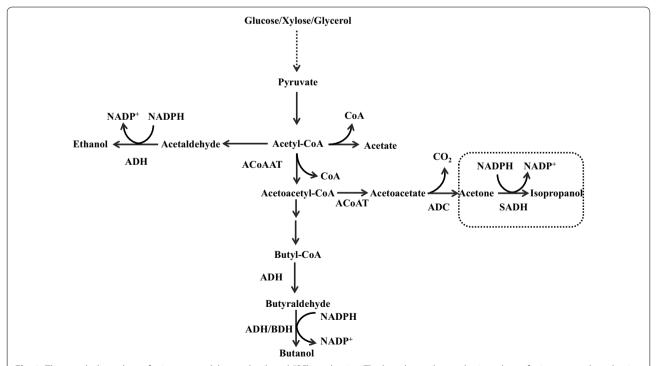
**Fig. 1** The metabolic pathway for isopropanol–butanol–ethanol (IBE) production. The box shows the synthetic pathway for isopropanol production from acetone. *ACoAAT* acetyl-CoA acetyl-transferase, *ACoAT* acetoacetyl-CoA transferase, *ADC* acetoacetate decarboxylase, *SADH* secondary alcohol dehydrogenase, *ADH* alcohol dehydrogenase, *BDH* butanol dehydrogenase
