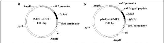
**Fig. 1** Schematic diagrams of the plasmids for expressing *DsRed*. **a** The pCbh1-DsRed plasmid for expressing *DsRed* intracellularly. **b** The pDsRed-AfMP1 plasmid for displaying *DsRed* on *T. reesei* cell surface. For both plasmids, the strong inductive *cbh1* promoter was used. *Af*MP1: the C-terminal GPI anchor from the *A. fumigatus* MP1 protein
