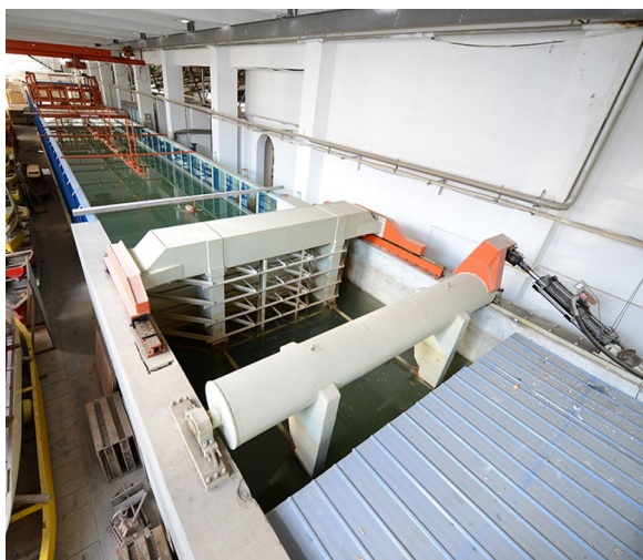
Fig. 2 Diagram showing the water tank that used for testing the hydrodynamics of floating PBRs
