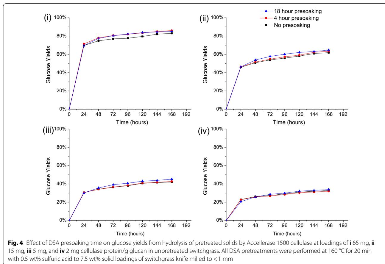
**Fig. 4** Effect of DSA presoaking time on glucose yields from hydrolysis of pretreated solids by Accellerase 1500 cellulase at loadings of **i** 65 mg, **ii** 15 mg, **iii** 5 mg, and **iv** 2 mg cellulase protein/g glucan in unpretreated switchgrass. All DSA pretreatments were performed at 160 °C for 20 min with 0.5 wt% sulfuric acid to 7.5 wt% solid loadings of switchgrass knife milled to < 1 mm
