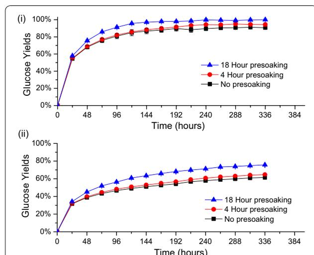
**Fig. 5** Effect of presoaking time on glucose yields from enzymatic hydrolysis of CELF pretreated by Accellerase 1500 cellulase at loadings of **i** 5 mg protein/g glucan in unpretreated switchgrass and **ii** 2 mg protein/g glucan in unpretreated switchgrass. All CELF pretreatments were performed at 150 °C for 25 min with 0.5 wt% sulfuric acid and a 0.889:1 THF/water mass ratio to 7.5 wt% solid loadings of switchgrass knife milled to < 1 mm
