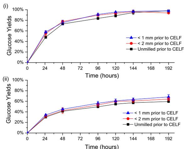
**Fig. 7** Effect of milling (particle size) on glucose yields from CELF-pretreated solids for enzymatic hydrolysis with Accellerase 1500 at cellulase loadings of **i** 5 mg and **ii** 2 mg cellulase protein/g glucan in unpretreated switchgrass. All CELF pretreatments were performed at 150 °C for 25 min with 0.5 wt% sulfuric acid and a 0.889:1 THF/water mass ratio for switchgrass that had first been presoaked for 18 h at 4 °C and a 7.5 wt% solids loading
