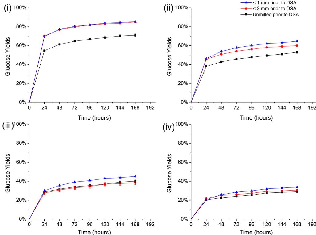
**Fig. 6** Effect of milling (particle size) on enzymatic glucose yields for pretreated solids prepared by DSA at Accellerase 1500 cellulase loadings of **i** 65 mg, **ii** 15 mg, **iii** 5 mg, and **iv** 2 mg cellulase protein/g glucan in unpretreated switchgrass. All DSA pretreatments were performed at 160 °C for 20 min with 0.5 wt% sulfuric acid on switchgrass that had first been presoaked for 18 h at 4 °C at a 7.5 wt% solids loading
