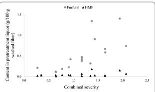
**Fig. 2** Furfural and HMF contents in the pretreatment liquor after steam pretreatment of the fiber fraction of animal bedding
