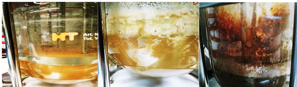
Fig. 6 Wall growth and biofilm formation in continuous A. succinogenes culture at the beginning of fermentation (left), during feeding with commercial sugars (middle) and during feeding with OFMSW hydrolysate (right)
