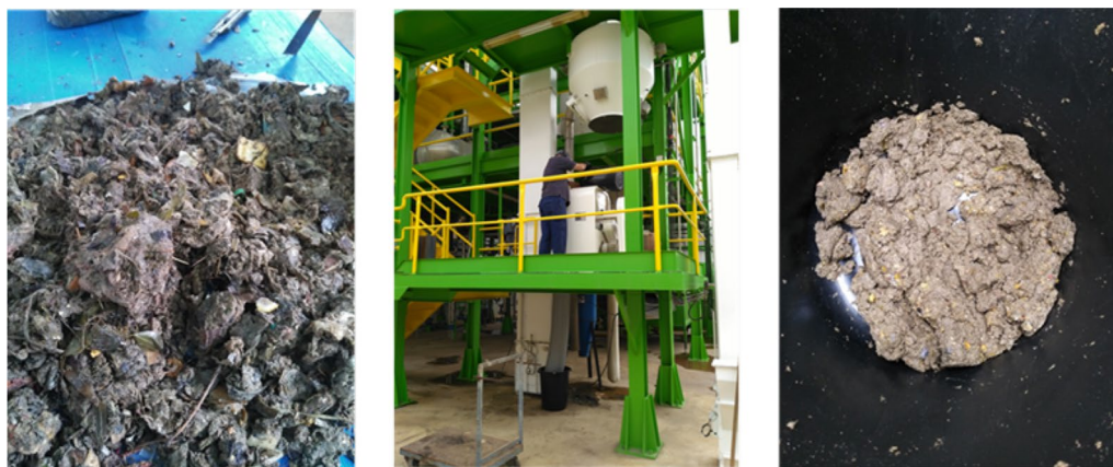
Fig. 8 OFMSW sample from MSW treatment plant after inert materials removal (left), milling facilities in IMECAL's pilot plant (middle), homogenized OFMSW sample after milling (right) ready for characterization and hydrolysis
