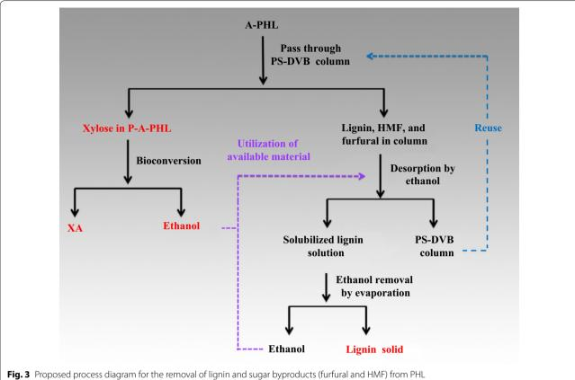
the regenerated resin can be reused in another purification process to adsorb the lignin and sugar byproducts in A-PHL. Hence, the present concept for the purification of A-PHL by PS-DVB resin is inherently environmentally friendly and sustainable.
