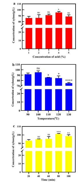
**Fig. 2** Effects of the acid concentration (**a**), temperature (**b**), and reaction time (**c**) of acid hydrolysis on xylose production [(**a**: temperature:  $100 \,^{\circ}$ C; time:  $60 \,^{\circ}$ min), (**b**: acid concentration: 4%; time:  $60 \,^{\circ}$ min), (**c**: acid concentration: 4%; temperature:  $100 \,^{\circ}$ C)]; ns denotes no significant difference, \* denotes p < 0.05, \*\* denotes p < 0.01 and \*\*\* denotes p < 0.001, \*\*\*\* denotes p < 0.0001
