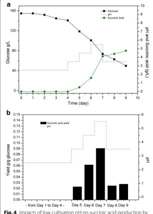
**Fig. 4** Impacts of low cultivation pH on succinic acid production by the SAP-3 strain at 35 °C. **a** Glucose consumption and succinic acid production (g/L); **b** yield of succinic acid at different pH levels
