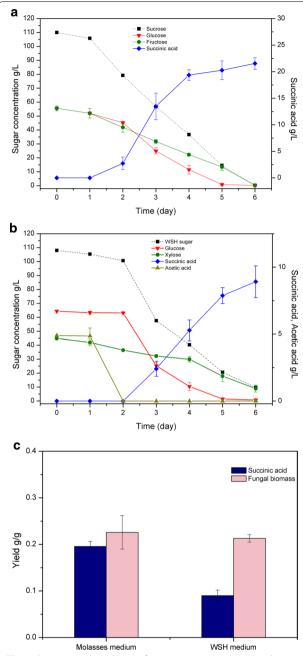
**Fig. 5** Succinic acid production from sugar cane molasses and wheat straw hydrolysate by the SAP-3 strain 35 °C. **a** succinic acid production and consumption of major sugars in sugar beet molasses; **b** succinic acid production and consumption of major sugars and acetic acid in wheat straw hydrolysate; **c** yields of succinic acids and fungal biomass (WSH—wheat straw hydrolysate)
