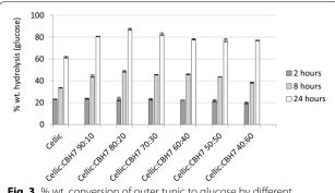
**Fig. 3** % wt. conversion of outer tunic to glucose by different combinations of Cellic CTec2 and CBHI. The total enzyme load was kept constant through the evaluation of the different combinations of Cellic CTec2 and CBHI
