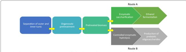
**Fig. 1** Flow diagram of the novel processes suggested for the valorisation of outer tunic. The valorisation flow diagram of outer tunic fraction towards bioethanol (*Route A*) and cellulose-derived oligosaccharides with prebiotic potential (*Route B*)
