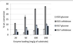
**Fig. 5** Mode of action of endoglucanase EG5 and EG7 on outer tunic. % wt. conversion of the substrate to glucose and cellobiose as a result of the effect of EG5 and EG7 action. The latter is a disaccharide with potential prebiotic activity
