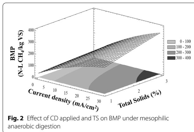
**Fig. 2** Effect of CD applied and TS on BMP under mesophilic anaerobic digestion
