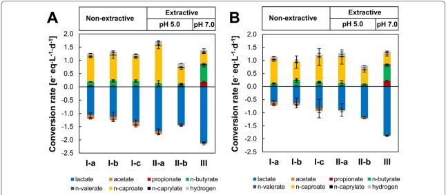
**Fig. 2** Conversion rates in (non-)extractive chain elongation continuous reactors: **A** R1 and **B** R2. Initial substrates were L-lactate and acetate. Conversion rates include carboxylates in aqueous and organic phases normalized to reactors working volume. Error bars show  $\pm$  one standard deviation except for periods II-a and III for which absolute deviation is shown
