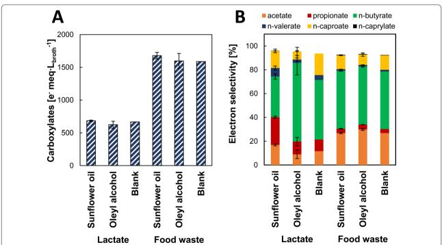
**Fig. 1** A Total carboxylates produced and **B** product selectivity from lactate and food waste (non-)extractive 20-day batch fermentation. Carboxylates partitioned in the organic and aqueous phases were added up and normalized to the initial aqueous phase (fermentation broth) volume. Error bars depict duplicates absolute deviation from the average
