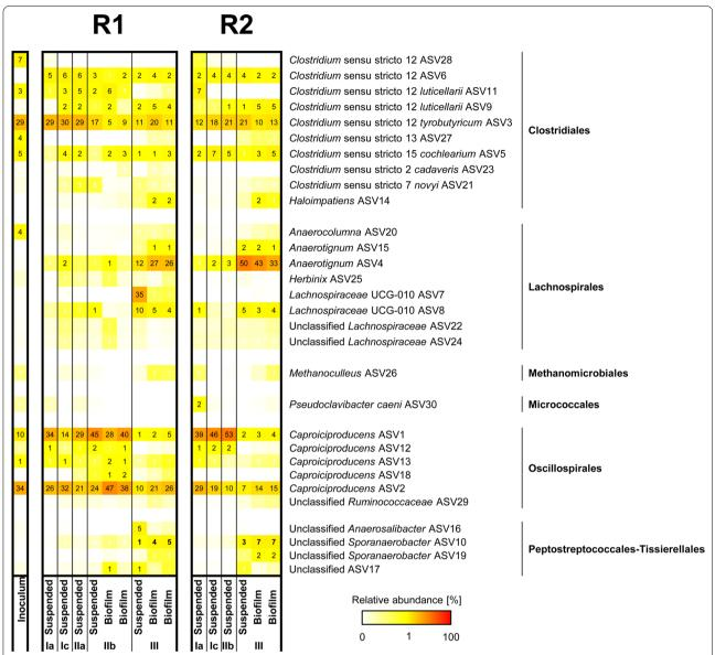
Fig. 4 Microbial community composition in (non-)extractive chain elongation continuous reactors at ASV level. Initial substrates were ∟-lactate and acetate. Top 30 ASVs are displayed and relative abundance values ≥ 1% are shown. Independent biofilm samples were analysed and shown as duplicates. Sampling days are shown in Additional file 1: Fig. S4. Taxonomy was assigned based on SILVA 138 SSU Ref NR 99 database
