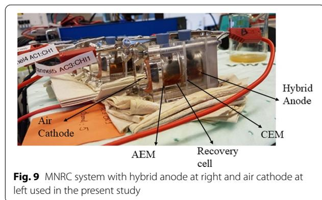
**Fig. 9** MNRC system with hybrid anode at right and air cathode at left used in the present study
