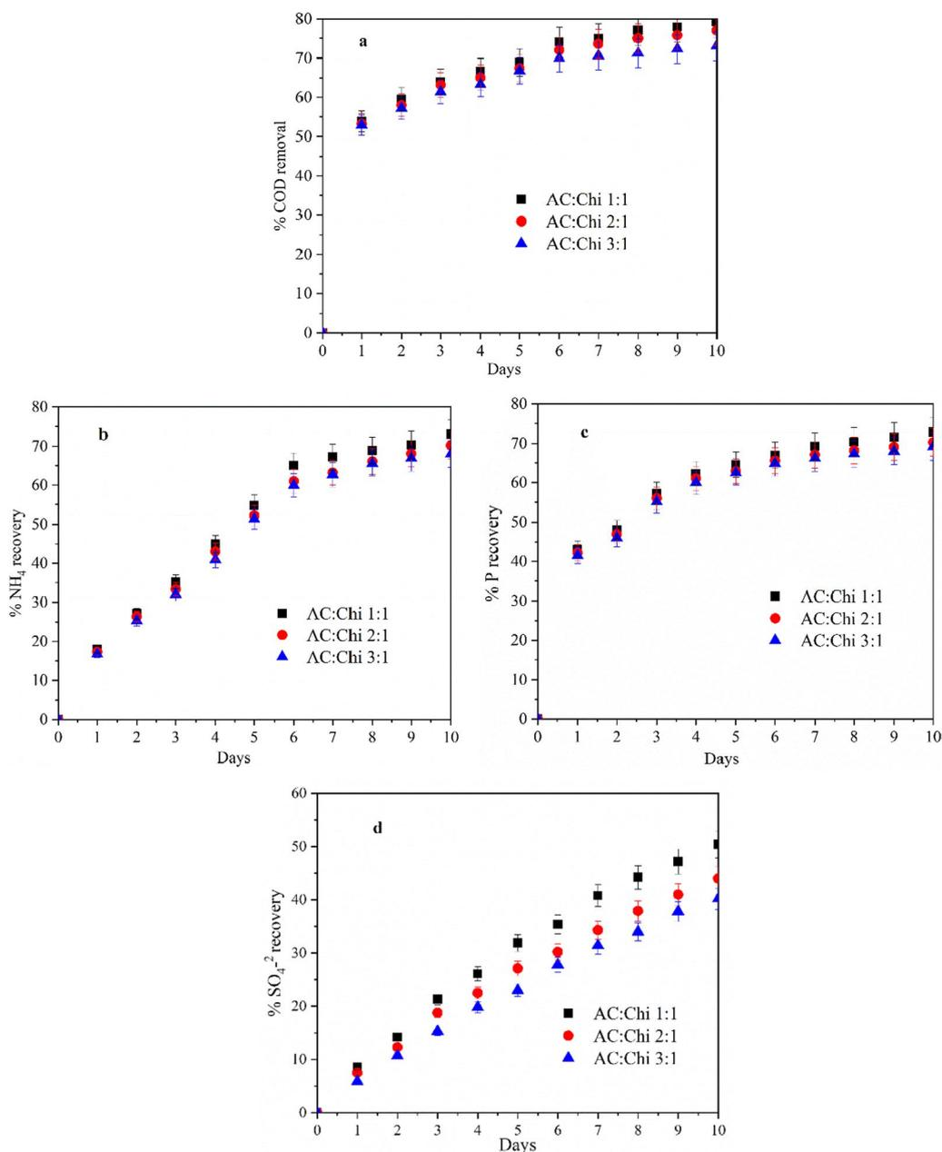
**Fig. 4** a COD removal, b % total phosphorus (P) recovery c % ammonium recovery, and d % SO<sub>4</sub><sup>2-</sup> recovery for hybrid anodes in the MNRC system for 10 cycles (i.e., 10 days of operation)
