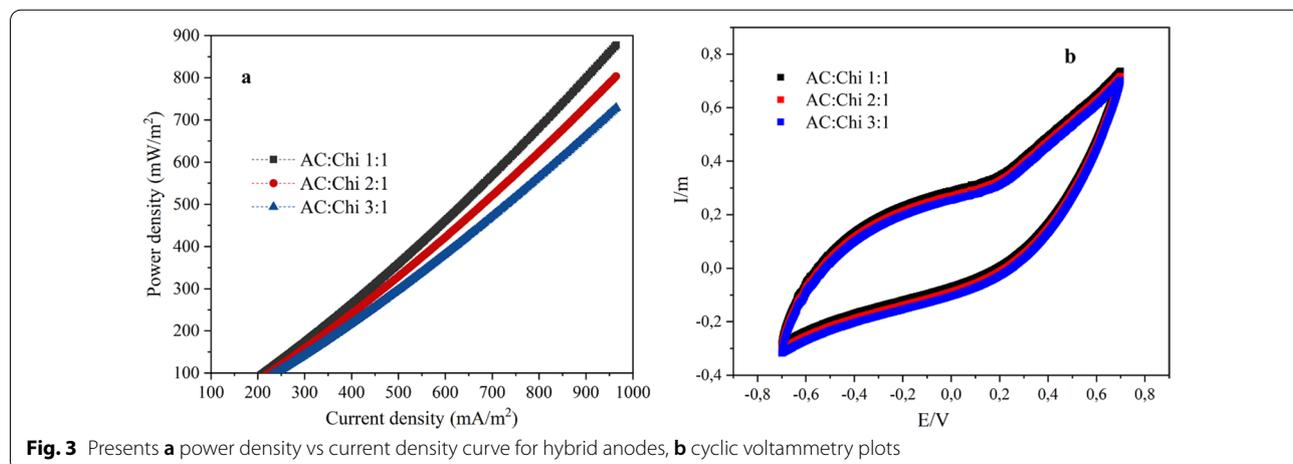
the presence of wastewater and potentiostat settings on the bioelectrochemical behavior of the systems was also investigated. Different forms and patterns of cyclic voltammograms were produced for the three hybrid anodes, as illustrated in Fig. 3b. Because of the varied electrode compositions and conductivities in the presence of wastewater, such discrepancies in the patterns were predicted.
